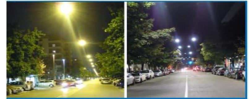
Example of a Milan neighborhood before (left) and after (right) conversion to LED street lighting. Source: communication with Municipality of Milano
