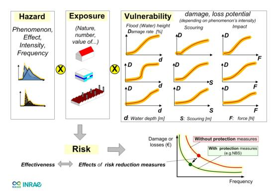
**Figure 6-1.** Basic components of risk: the effectiveness of a risk reduction measure requires to analyse its effects on the phenomenon including (1) the nature of the effects (e.g., flooding, scouring, impact of boulders); (2) their frequency; and (3) their intensity (e.g., flood depth) and their interaction with exposed elements (exposure and vulnerability as a potential of damage).
