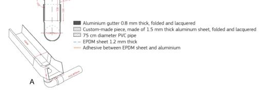
Figure 5-8. URBAN GreenUP Project: Green Façade construction details (© SingularGreen).
