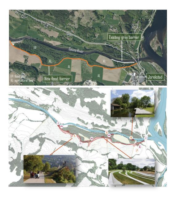
Figure 6-11. Aerial photo of the area with the location of the existing flood barrier and the new flood barrier (top); Visualization of the area with the potential multiple actions that can be supported by the flood barrier (by AgenceTer, bottom).
