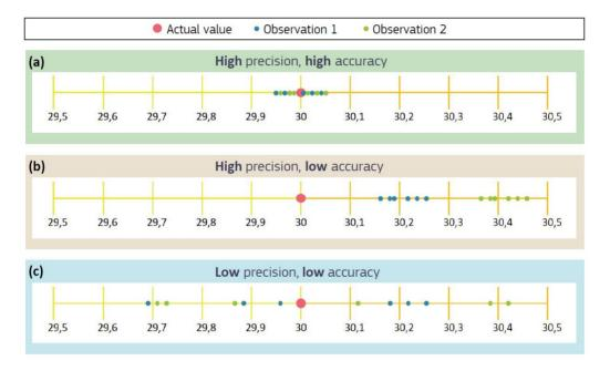
**Figure 7-9.** Measurements obtained with a temperature sensor which has (a) high precision and high accuracy (good quality sensor); (b) high precision bur low accuracy; (c) low precision and low accuracy (low quality sensor). The red dot represents the actual ("true") value of temperate. The blue and green dots represent the first sample collection (Observation 1) and second sample collection (Observation 2) respectively.
